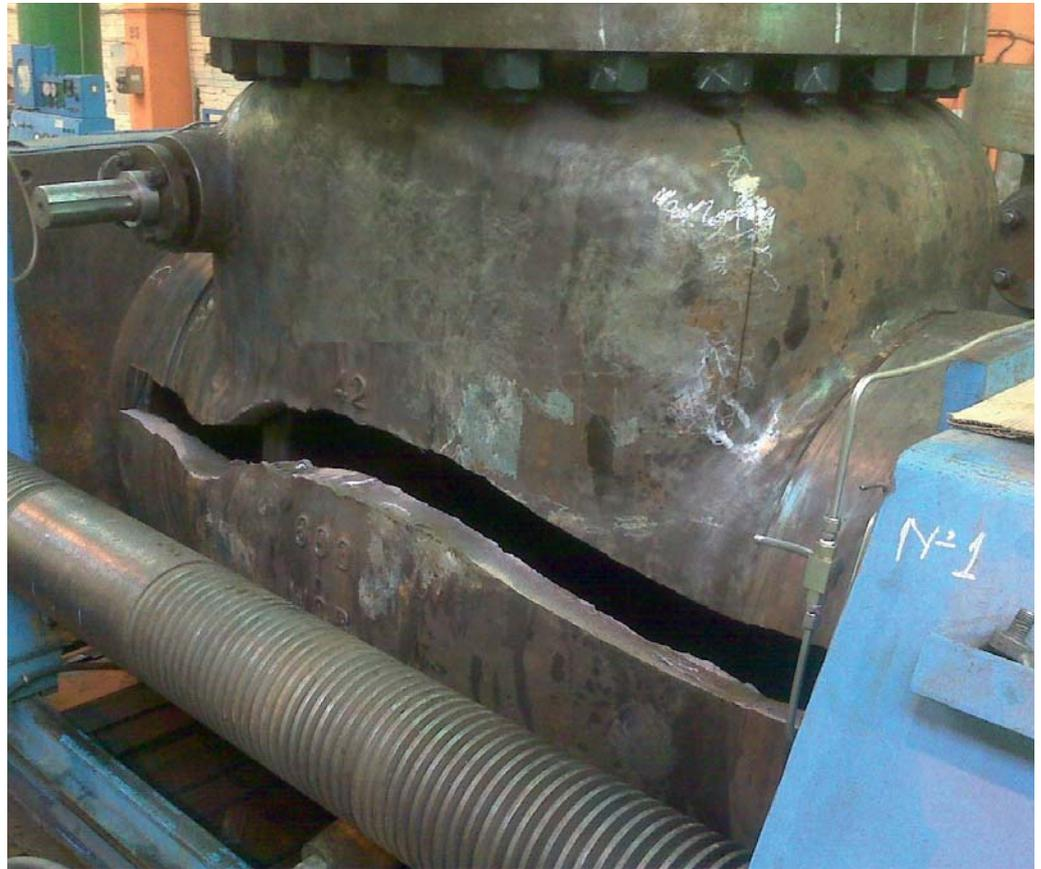
*This check valve broke during pressure testing*
